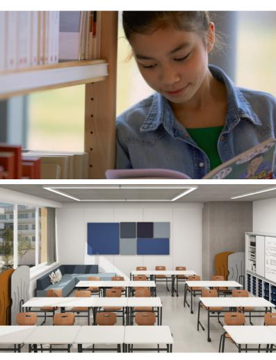
**Fabric-covered wall elements.** Thanks to maximum absorption performance ( $\alpha_w = 1$ ), the fabric-covered wall elements absorb a lot of sound even with a small surface area. Different sizes and fabric colors allow them to be cleverly integrated into any learning area; and thanks to sturdy edges and washable covers, they are particularly durable as well.
